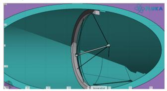
However, since about 10% of the 7.3 kW proton beam power are deposited into the target, a more sophisticated design was needed to allow for sufficient radiative cooling of the target, so that it survives a full year of Mu2e running.
