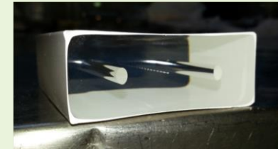
4 overlapping layers of scintillator bars with 2 wavelength-shifting fibers
